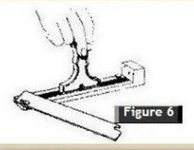
Slide and adjust type in adapter using scale provided for centering or line-up purposes.
