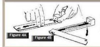
Lay adapter face down on a flat surface, Figure 4A.
