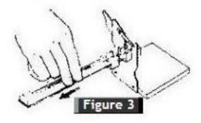
Remove adapter from cutting device
