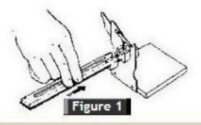
Adapter is attached to type cutting device by inserting pins into holes of adapter as shown in Figure 1.
